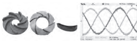
Fig. 2. (a) Components of AFSPM, (b) Back-emf at 1000 rpm
