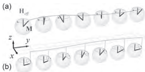
Fig. 1. (a) The precession spin wave without inertia (red curve). The blue arrow indicates the motion of the magnetization M . (b) The nutation surface spin wave (purple curve) with a frequency considerably higher than in (a) plotted with small blue circles on top of the “frozen” precession motion.
