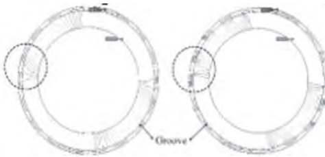
Fig. 2 Magnetic flux line before(a) and after(b) ferrofluid injection of multiple groove type model
