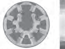
Fig. 2. No-load flux distributions when the stator DC/AC current is 14/0 A, rotor current is 0A.
