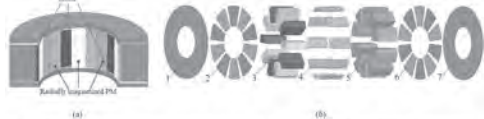
Fig. 7: Model 2: (a) Rotor structure of Model 2. (b) Details of the pole 1 and 7 are the rotor yoke, 2 and 6 are axially magnetized PM, 3 is the tangentially magnetized PM, 4 is the radially magnetized PM, 5 is the rotor.
