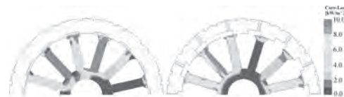
Fig. 5 Stator core loss distributions of the FMPM motors. (a) Stator core loss of the surface-insert FMPM motor. (b) Stator core loss of the spoke-type FMPM motor.
