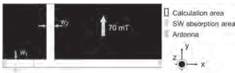
Fig.1. Overview of the calculation area. SWs are excited at the orange area.
