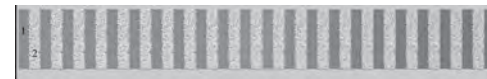
Fig. 1 Schematic of the nanowire with two different magnetic materials. The red vertical stripe in (1) is NiFe and the gray (2) is CoFe.
