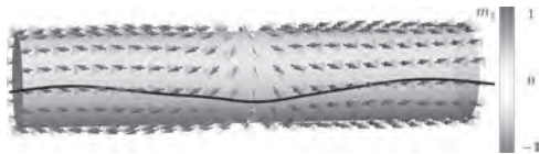
Fig. 1. A ferromagnetic nanotube with a domain wall possessing a finite Skyrmion charge. The arrows represent magnetizations of spin-wave excitations. The black curve lines the heads of the arrows. The axis of the nanotube is the z -axis.
