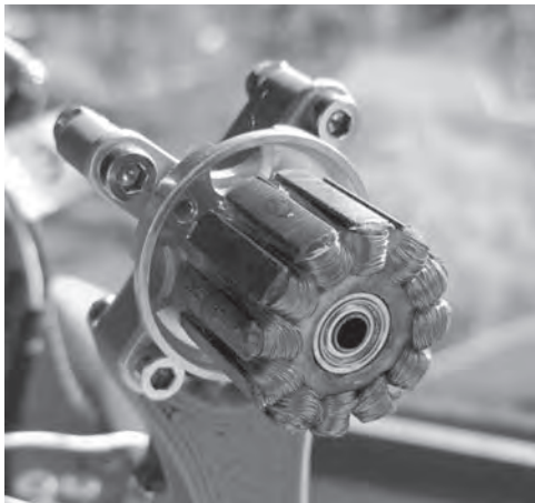
Fig. 2 A photo of the nanocrystalline (\text{Fe}_{0.8}\text{Co}_{0.2})_{86}\text{B}_{14} electric motor stator core produced by CURA after winding of the excitation coils and mounting to a commercially available 220 W motor frame.
