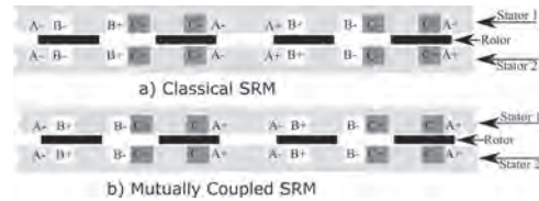
Fig.1 Winding configuration of the AFDSRM, a) Classical winding, b) Mutually coupled.
