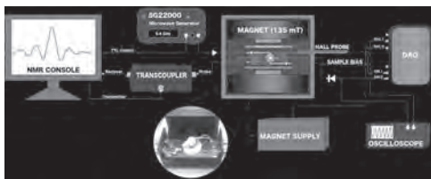
Fig. 1. Schematic of the table-top MRI system showing NMR and hyperpolarizer systems along with a photo of the 3 mm diameter NMR cell and hyperpolarizer, contained in a 25 mm x 50 mm enclosure.
