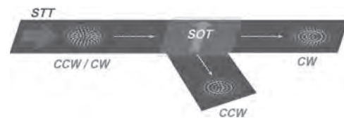
Figure 1. Illustration of a nanowire with a branch to discriminate a skyrmion chirality.
