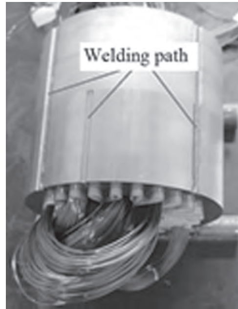
Fig. 2 Fixing process of conventional core
