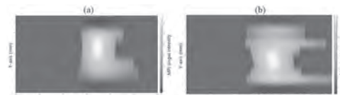
MPI signal intensity and spatial distribution of the commercial MPI tracers: (a) Perimag, (b) Vivotrax Plus.
