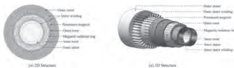
Schematic diagram of the proposed LSHTM with single hybrid rotor and double stator
