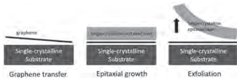
Fig. 1 Schematic illustration of remote epitaxy process of single-crystalline complex-oxide materials.
