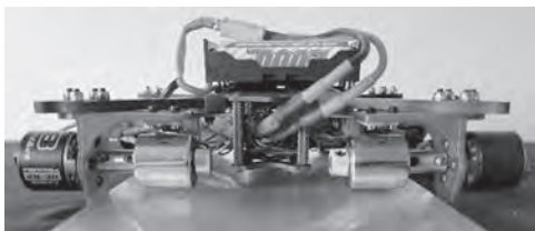
Fig. 1. The four rotor, one-pole pair, wirelessly controlled proof-of-principle, EDW maglev drone shown placed above a 6061 grade aluminum track that is 9.5mm thick and 152mm wide.
